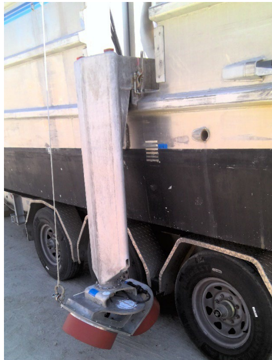
Figure 6: R/V Benthos MBES sonar heads over-the-side mount during dimensional control survey March 2021.
